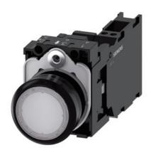
Illuminated pushbutton, 22 mm, round, plastic, white, pushbutton, flat, momentary contact type, with holder, 1 NO+1 NC, LED module with integrated LED 230 V AC, spring-type terminal, with laser labeling, upper case
