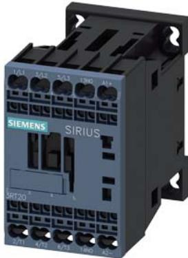
traction contactor, AC-3e/AC-3, 16 A, 7.5 kW / 400 V, 1 NO, 72-125 V DC, 0.7-1.25\*Us with integrated varistor frame size S00, spring-loaded terminal suitable for PLC outputs
