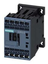
power contactor, AC-3 12 A, 5.5 kW / 400 V 1 NO, 24 V DC 0.7-1.25\*US 3-  $\,$ pole, size S00 spring-type terminal suitable for PLC outputs not expandable with auxiliary switch
