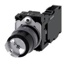
RONIS key-operated switch, 22 mm, round, plastic with metal front ring, lock number SB30, with 2 keys, 2 switch positions O-I, latching, actuating angle 90°, 10:30h/13:30h, key removal O+I, with holder, 1 NO+1 NC, screw terminal, possible special locks: SB31, 421, 455, with laser labeling, upper case and lower case, always upper case at the beginning of the word
