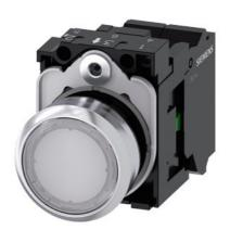
Illuminated pushbutton, 22 mm, round, metal, shiny, white, pushbutton, flat, momentary contact type, with holder, 1NO, LED module with integrated LED 110 V AC, spring-type terminal, with laser labeling, inscription or symbol Customer-specific selection with SIRIUS ACT configurator (CIN)
