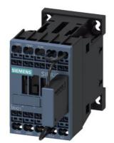
Contactor relay for railway, 2 NO + 2 NC DC 72 V, 0.7 ... 1.25\* US, with integrated suppressor diode, Size S00, Spring-type terminal suitable for PLC outputs
