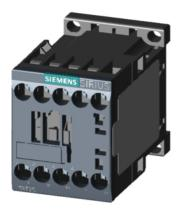
Power contactor, AC-3 12 A, 5.5 kW / 400 V 2 NO + 2 NC 48 V AC, 50/60 Hz 4-pole Size S00 screw terminals
