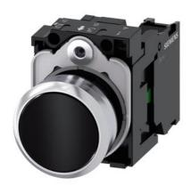
Pushbutton, 22 mm, round, metal, shiny, black, pushbutton, flat, momentary contact type, with holder, 1 NO, screw terminal, with laser labeling, inscription or symbol Customer-specific selection with SIRIUS ACT configurator (CIN)
