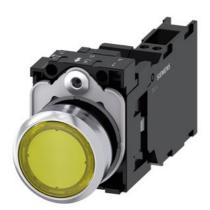
Illuminated pushbutton, 22 mm, round, metal, shiny, yellow, pushbutton, flat, momentary contact type, with holder, 1 NO+1 NC, LED module with integrated LED 110 V AC, spring-type terminal, with laser labeling, inscription or symbol Customer-specific selection with SIRIUS ACT configurator (CIN)
