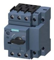
Circuit breaker size S00 for motor protection, CLASS 10 with overload relay function A-release 3.5...5 A N release 65 A screw terminal Standard switching capacity
