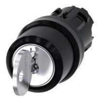
RONIS key-operated switch, 22 mm, round, plastic, lock number SB30, with 2 keys, 3 switch positions I-O-II, latching, actuating angle 2x45°, 10:30h/12h/13:30h, Key removal II, possible special locks: SB31, 421, 455, with laser labeling, inscription or symbol Customer-specific selection with SIRIUS ACT configurator (CIN)
