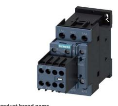
Power contactor, AC-3 32 A, 15 kW / 400 V 2 NO + 2 NC, 400 V AC, 50 Hz 3-pole, size S0 screw terminals Removable auxiliary switch
