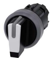
Selector switch, illuminable, 22 mm, round, plastic with metal front ring, white, selector switch, short, 3 switch positions I>O<II, momentary contact on the left, latching on the right, actuating angle  $2x45^{\circ}$ , 10:30h/12h/13:30h, with laser labeling, upper case
