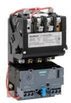
Non-reversing motor starter, Size 0, Three phase full voltage, Solid-state overload relay, OLRelay amp range 5.5-22a, 24Vdc coil, Non-combination type, Enclosure type (open), No enclosure
