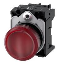
Indicator lights, 22 mm, round, plastic, red, lens, smooth, with holder, LED module, with integrated LED 230 V AC, screw terminal  $\,$
