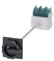
SENTRON, Switch disconnector 3LD, main switch, 3-pole, lu: 100 A, Operating power / at AC-23 A at 400 V: 37 kW, floor mounting with door coupling, rotary operating mechanism, black, 4-hole mounting of the handle
