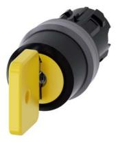
Key-operated switch O.M.R, 22 mm, round, plastic with metal front ring, lock number 73033, yellow, with 2 keys, 3 switch positions I-O-II, latching, actuating angle 2x45°, 10:30h/12h/13:30h, Key removal I+O+II, Z=50-unit packaging
