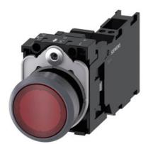
Illuminated pushbutton, 22 mm, round, plastic with metal front ring, red, pushbutton, flat, momentary contact type, with holder, 1 NO+1 NC, LED module with integrated LED 24 V AC/DC, spring-type terminal, with laser labeling, upper case
