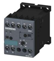
Timing relay, electronic Multifunction, 8 functions 1 change-over contact 24 V AC/DC, 200 to 240 V AC at 50/60 Hz AC 0.05 s to 100 h Overall width 45 mm screw terminal
