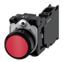
Pushbutton, 22 mm, round, plastic, red, pushbutton, flat, momentary contact type, with holder 1 NO+1 NC, spring-type terminal, with laser labeling, lower case
