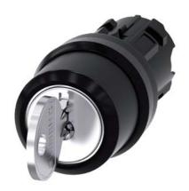
RONIS key-operated switch, 22 mm, round, plastic, lock number SB30, with 2 keys, 3 switch positions I-O-II, latching, actuating angle 2x45°, 10:30h/12h/13:30h, key removal O+I, possible special locks: SB31, 421, 455 Z=50-unit packaging
