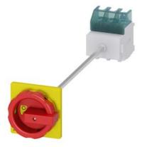
SENTRON, Switch disconnector 3LD, emergency switching-off switch, 3-pole, Iu: 63 A, operating power / at AC-23 A 400 V: 22 kW, floor mounting with door coupling, rotary operating mechanism, Red / yellow, 4-hole mounting of the handle
