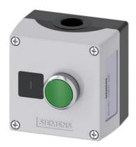
Enclosure for command devices, 22 mm, round, Enclosure material metal, enclosure top part gray, 1 control point metal, A=Pushbutton green, 1 NO, screw terminal, floor mounting, label: I, 1xM20 each on top and bottom, I abel enclosed
