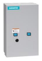
2-speed 3-phase motor starter, Size 0, Two separate windings, Constant horsepower, Solid-state overload relays, Low Spd OLR range 0.75-3.4A, High Spd OLR range 0.75-3.4A, 110V 50Hz / 120V 60Hz coil, Enclosure NEMA type 1, Indoor general purpose use
