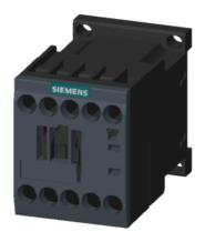
Power contactor, AC-3 9 A, 4 kW / 400 V 1 NC, 120 V AC, 50 / 60 Hz 3-pole, Size S00 screw terminal
