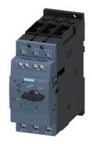
Circuit breaker size S2 for motor protection, CLASS 10 A-release 14...20 A N-release 260 A screw terminal Standard switching capacity with transverse auxiliary switches 1 NO+1 NC
