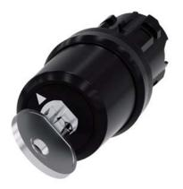
key-operated switch Siemens, 22 mm, round, plastic, lock no. LSG1, with 2 keys, 2 switch positions O-I, latching, actuating angle  $90^\circ,\,10:\!30h/13:\!30h,$  key removal O+I, with laser labeling, lower case
