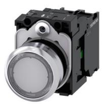
Illuminated pushbutton, 22 mm, round, metal, shiny, clear, pushbutton, flat, momentary contact type, with holder, 1NO, LED module with integrated LED 24 V AC/DC, screw terminal, with laser labeling, lower case
