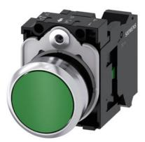
Pushbutton, 22 mm, round, metal, shiny, green, pushbutton, flat, momentary contact type, 1 NO, spring-type terminal, with laser labeling, upper case
