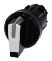
Selector switch, illuminable, 22 mm, round, plastic, white, selector switch, short, 3 switch positions I-O<II, left latching, right momentary contact type, actuating angle  $2x45^{\circ}$ , 10:30h/12h/13:30h, with laser labeling, upper case
