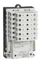
Electrically held lighting contactor, (convertible to mech. held), Amp rating 30A (tungsten 20A), 6 N.C. / 1 N.O. poles, 115-120V 60Hz/110V 50Hz coil, Non-combination type, Enclosure NEMA type (open), No enclosure
