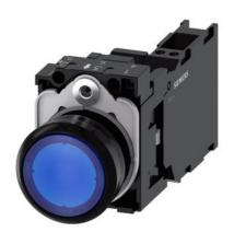
Illuminated pushbutton, 22 mm, round, plastic, blue, pushbutton, flat, momentary contact type, with holder, 1 NO+1 NC, LED module with integrated LED 110 V AC, spring-type terminal, with laser labeling, upper case and lower case, Always upper case at the beginning of the word
