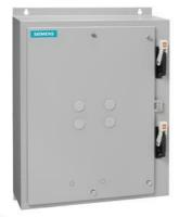
Duplex starter w/o alternator, Size 1, Three phase full voltage, Solid-state overload relay, OLR amp range 5.5-22A, 208VAC 60Hz coil, Combination type, Two 25A circuit breakers, Enc NEMA type 4 painted steel, Water/dust tight for outdoors
