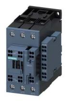
power contactor, AC-3 40 A, 18.5 kW / 400 V 2 NO + 2 NC, 110 V AC 50 Hz, 3-pole, Size S2, Spring-type terminal lateral auxiliary switch block
