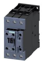
power contactor, AC-3 51 A, 22 kW / 400 V 1 NO + 1 NC, 24 V DC with varistor, 3-pole, size S2, screw terminal suitable for 2 A PLC outputs
