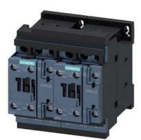
Reversing contactor assembly AC-3,11 kW/400 V,AC230V,50/60Hz 3-pole, Size S0 screw terminal electrical and mechanical Interlock 2 NO integrated
