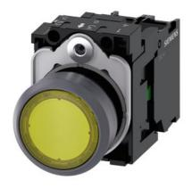
Illuminated pushbutton, 22 mm, round, plastic with metal front ring, yellow, pushbutton, flat, momentary contact type, with holder, 1 NO, LED module with integrated LED 110 V AC, screw terminal
