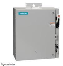
Pump control panel, Size 1, Three phase full voltage, Solid-state overload relay, OLR amp range 10-40A, 190-220/220-240V 50/60Hz coil, Standard type contactor, 30A circuit breaker, HOA Sel Sw. <(>&<)> Start P.B., Enclosure NEMA type 3/3R, Weather proof outdoor use
