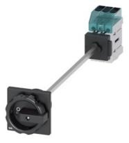
Load disconnector 3LD3, lu 16 A Main switch 3-pole Rated operating capacity at AC-23 A at 400V 7.5kW floor mounting Basic switch with door coupling Central hole mounting 22.5mm Rotating drive black 66 x 66 mm
