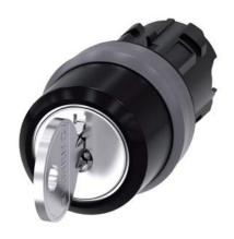
RONIS key-operated switch, 22 mm, round, plastic with metal front ring, lock number SB30, with 2 keys, 3 switch positions I-O<II, left latching, right momentary contact type, actuating angle  $2x45^{\circ}$ , 10:30h/12h/13:30h, key removal O, possible special locks: SB31, 421, 455, Z=50-unit packaging
