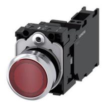
Illuminated pushbutton, 22 mm, round, metal, shiny, red, pushbutton, flat, momentary contact type, with holder, 1 NO+1 NC, LED module with integrated LED 110 V AC, spring-type terminal, with laser labeling, upper case and lower case, Always upper case at the beginning of the word
