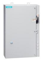
Non-reversing motor starter, Size 1 3/4, Three phase full voltage, Solid-state overload relay, OLR amp range 10-40A, 110V 50Hz / 120V 60Hz coil, Combination type, 60A fusible disconnect, 60A/250V fuse clip, Encl NEMA type 4X 304 S-Steel, Water/dust tight noncorrosive, Extra-wide enclosure
