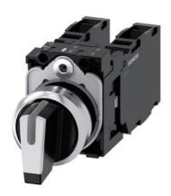
Selector switch, illuminable, 22 mm, round, metal, shiny, white, selector switch, short, 3 switch positions I>O<II, momentary contact type, actuating angle  $2x45^{\circ}$ , 10:30h/12h/13:30h, with holder, 2x1NO+1NC, screw terminal
