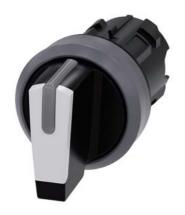
Selector switch, illuminable, 22 mm, round, plastic with metal front ring, white, selector switch, short, 3 switch positions I-O<II, left latching, right momentary contact type, actuating angle  $2x45^{\circ},\,10:30h/12h/13:30h$
