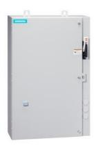
Non-reversing motor starter, Size 1, Three phase full voltage, Solid-state overload relay, OLR amp range 3-12A, 208VAC 60Hz coil, Combination type, 30A non-fusible disconnect, Encl NEMA type 4X 304 S-Steel, Water/dust tight noncorrosive, Extra-wide enclosure
