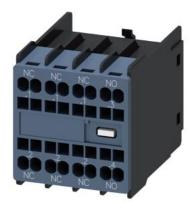
Auxiliary switch on the front, 1 NO + 3 NC Current path 1 NC, 1 NC, 1 NC, 1 NO, 1 NO for 3RH and 3RT spring-type terminal .1/.2, .1/.2, .1/.2, .3/.4
