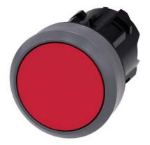
Pushbutton, 22 mm, round, plastic with metal front ring, red, pushbutton, flat, latching, Push-to-release mechanism, with laser labeling, upper case and lower case, always upper case at beginning of line
