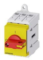
Load disconnector 3LD3, lu 16 A Main switch 3-pole Rated operating capacity at AC-23 A at 400V 7.5kW Installation in distribution boards, Basic switch with selector knob red / yellow
