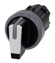
Selector switch, illuminable, 22 mm, round, plastic with metal front ring, white, selector switch, short, 3 switch positions I-O<II, left latching, right momentary contact type, actuating angle 2x45°, 10:30h/12h/13:30h, with laser labeling, upper case and lower case, always upper case at beginning of line
