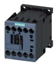
Power contactor, AC-3 16 A, 7.5 kW / 400 V 1 NO, 24 V DC communication-capable, 3-pole Size S00, screw terminals
